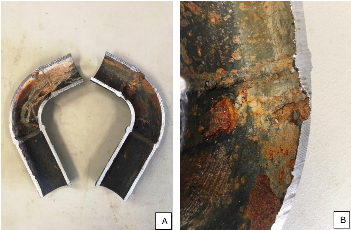
Picture A & B – 2" Pipe sample from the 17L-794 Well flowline before cleaning
