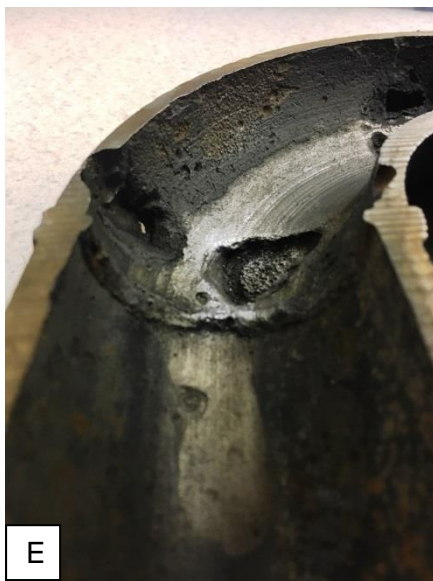
Pictures C, D, E & F show the exposed damage after HCl cleaning
