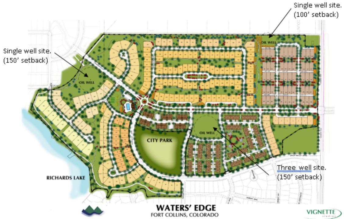
Fig 1 – Showing the Waters' Edge Subdivision with existing well sites and recommended setbacks.
