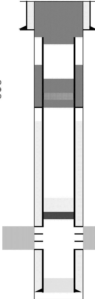
Cut surface casing off 6'-8' below surface.
