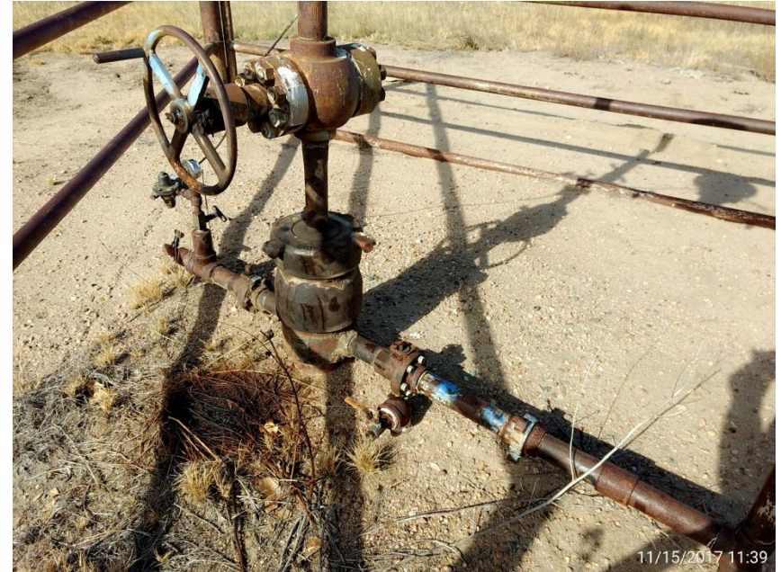
Wellhead detail, Corrective Action: Packing in master valve appears to be leaking causing stained soil.
