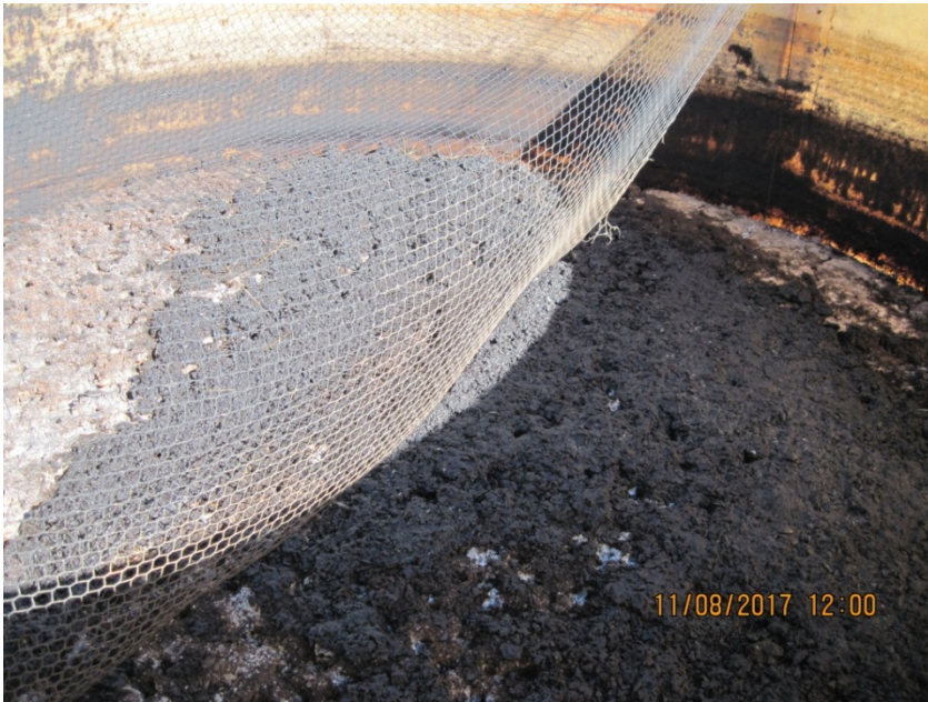
11. Inadequate wildlife netting with fluid in tank
