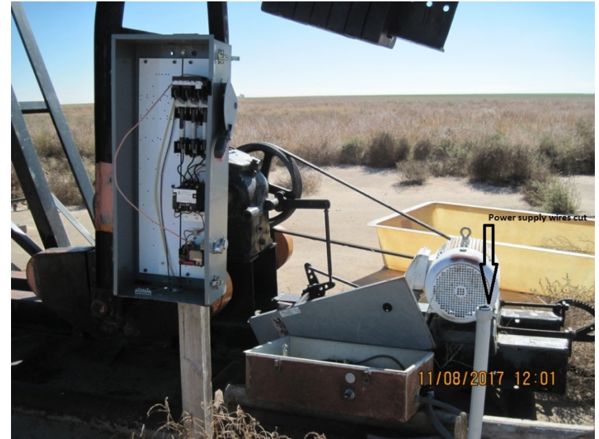
Incapable of producing in present state. Power supply cut off
