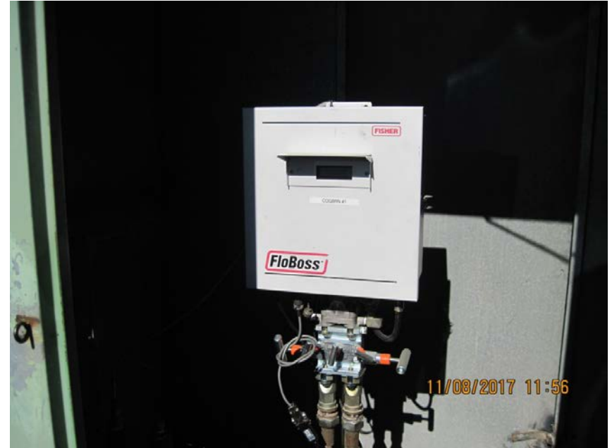
4. Electronic meter run
