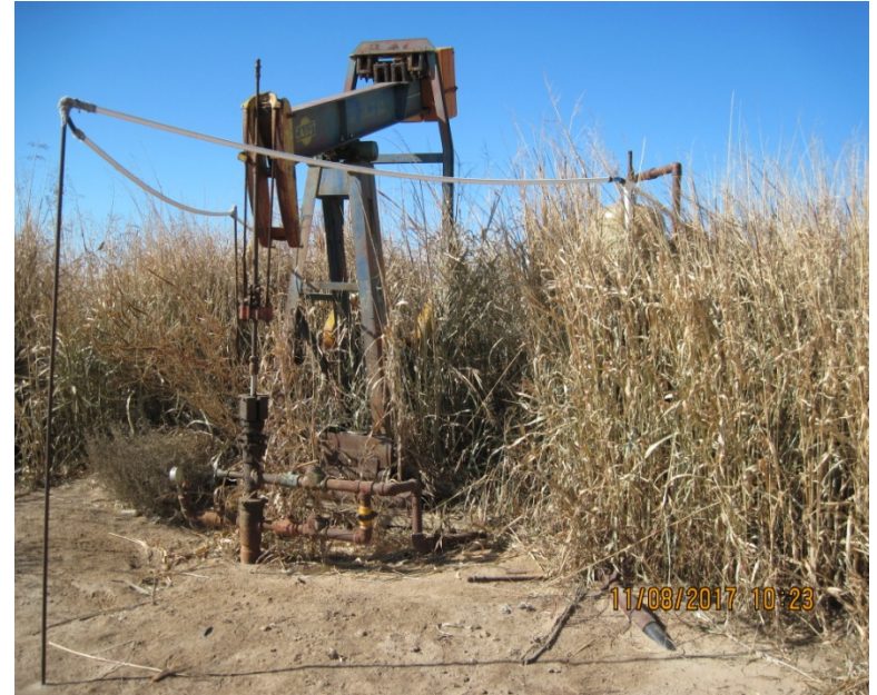
2. Pumping unit & VGS covered with vegetation 11/8/2017
