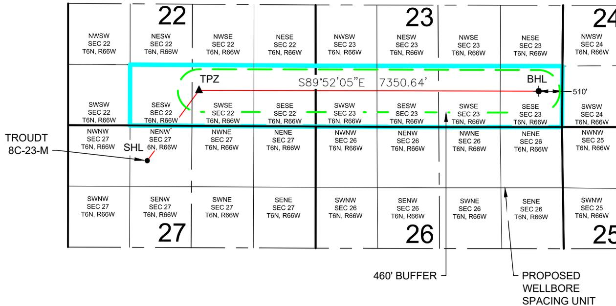
**TROUDT 8C-23-M WELL TO BE LOCATED 760' FNL AND 1715' FWL, SEC 27, T6N, R66W**
