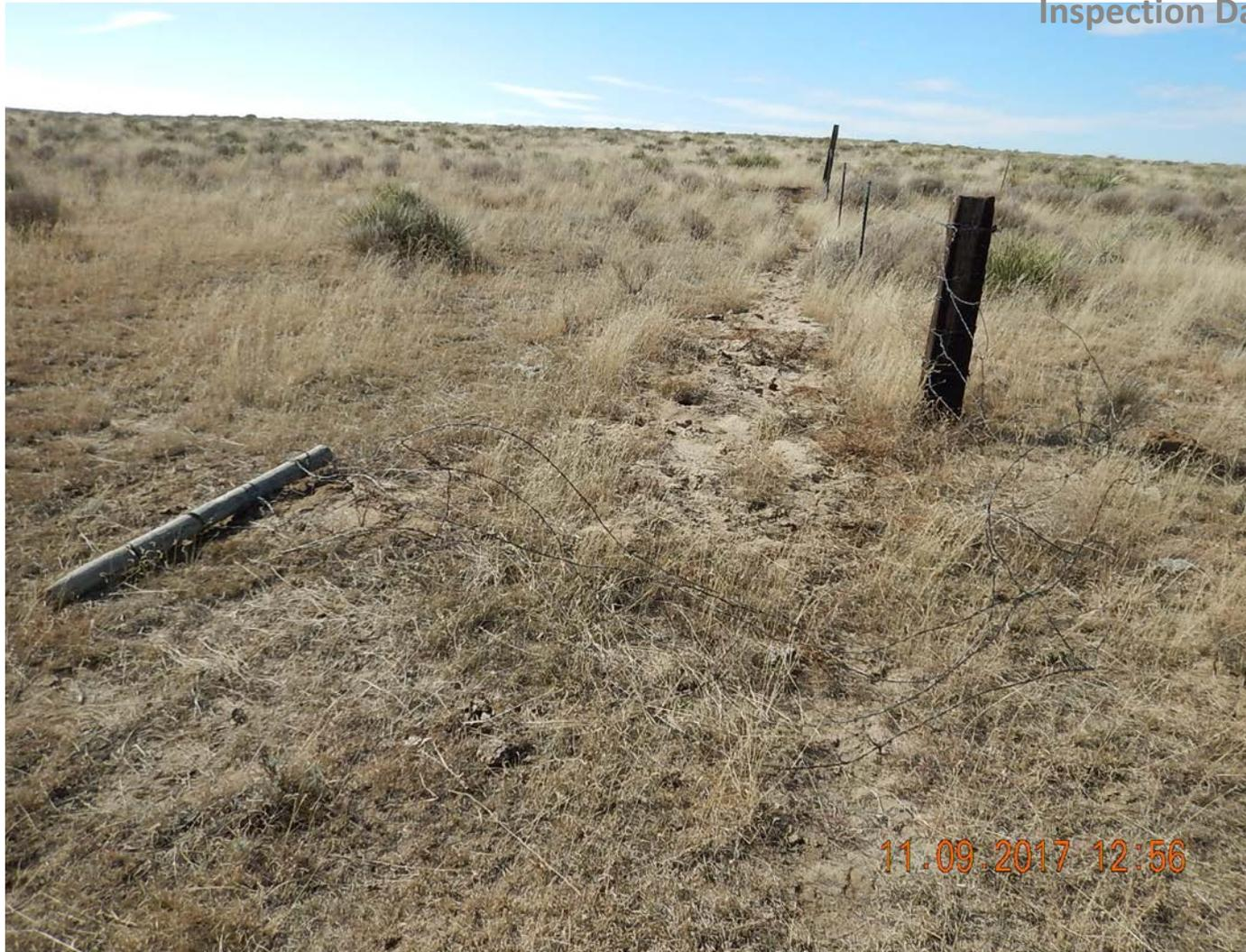
Gate on south side of well pad has not been repaired since previous inspection. Gate was down during inspection allowing cattle access to well pad.
