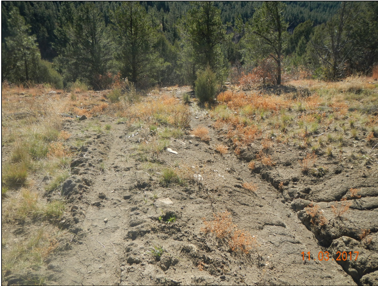
Photo 6. Facing toward the southwest side of the location. The ditch directs stormwater toward this direction however no other BMP's are installed to contain sediment and stormwater erosion.
