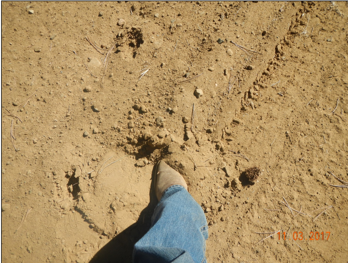
Photo 2. The soil pushed onto the road is loose and susceptible to erosion.
