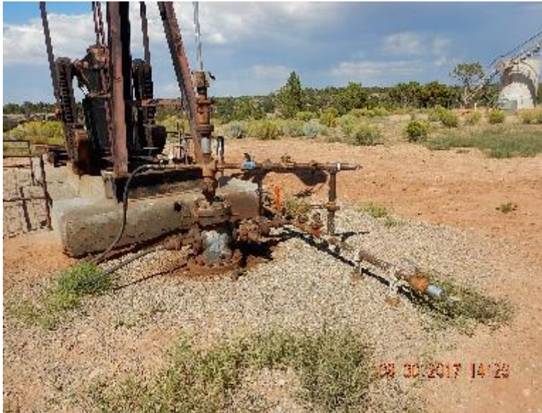
Photo 3: Wellhead with impacted soil around base of wellhead and 1" steel riser. Previous inspection.
