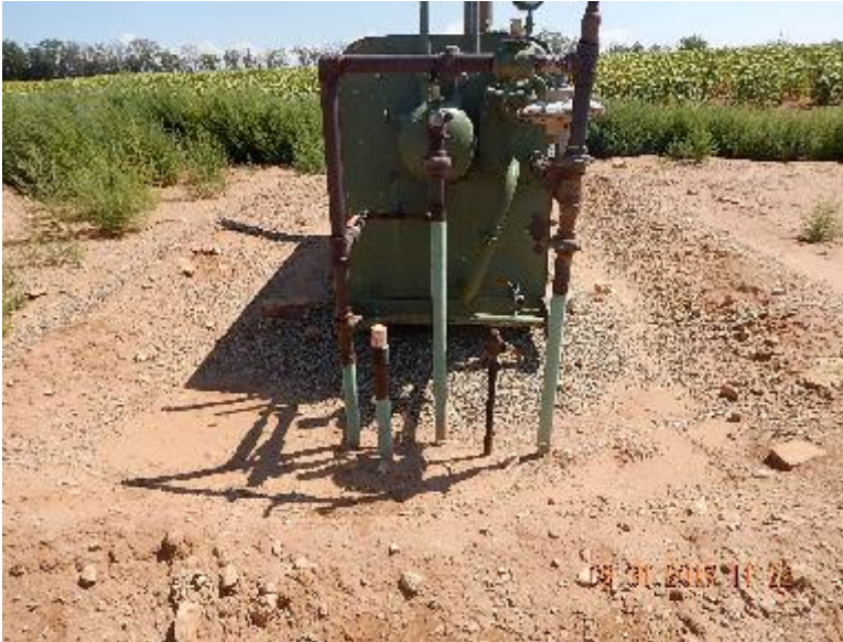
Photo 3: Disconnected risers at separator. Previous inspection.
