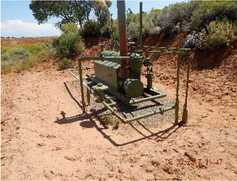
Photo 5: Separator and risers. Previous inspection.
