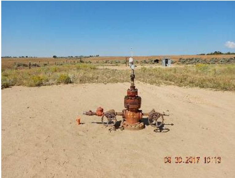
Photo 3: Disconnected wellhead and flowline riser. Previous inspection.
