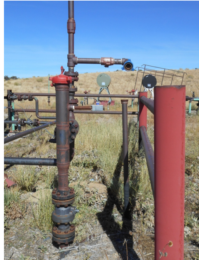
Abandoned risers not locked out/tagged out or marked for abandonment.
