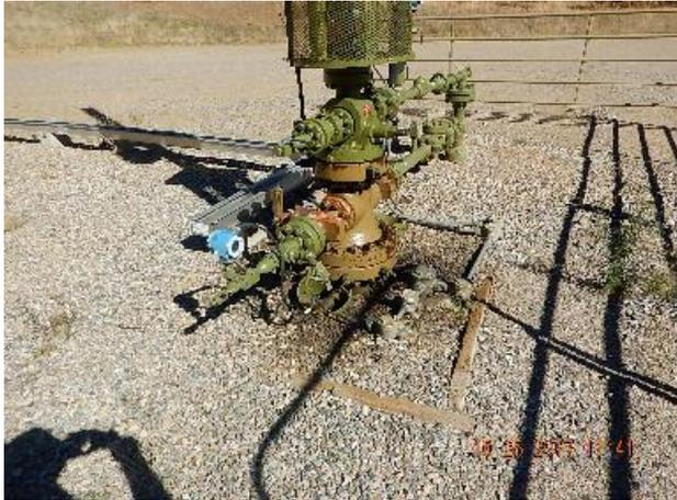
Photo 5: Impacted soil and gravel at base of wellhead.
