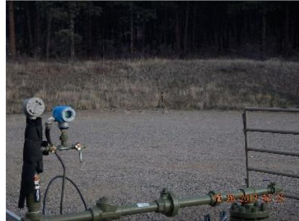
Photo 6: Sound meter set up 100' from wellhead on location.
