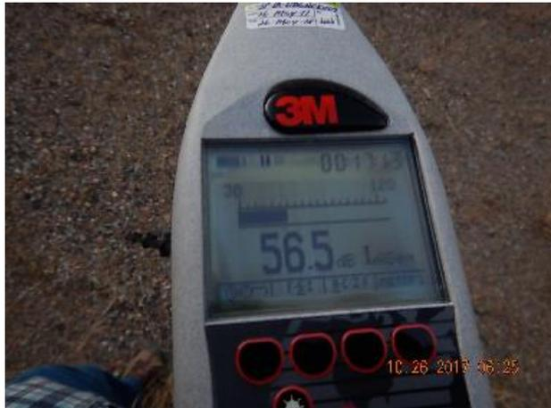
**Photo 7: Sound meter reading at test conclusion on location. Reading converts to 46.5 db(a) after plugging result into db(a) calculator.**
