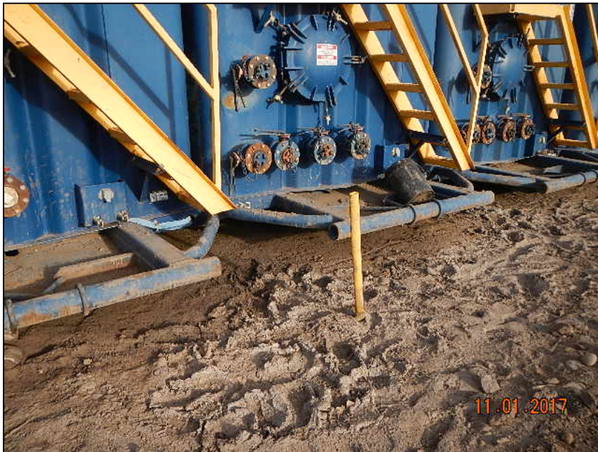
Photo 3. Staining under tanks.
