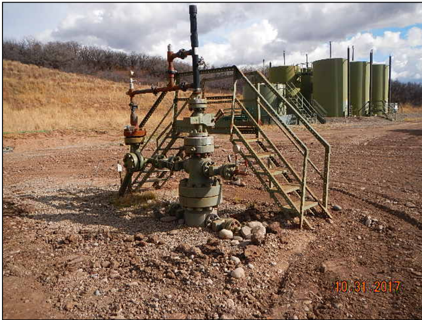
Photo 7. No sign at wellhead.
