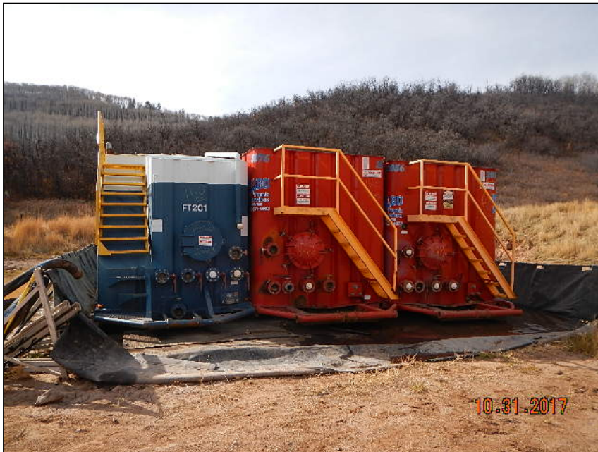
Photo 3. Frack tanks with no labels and containment not maintained.
