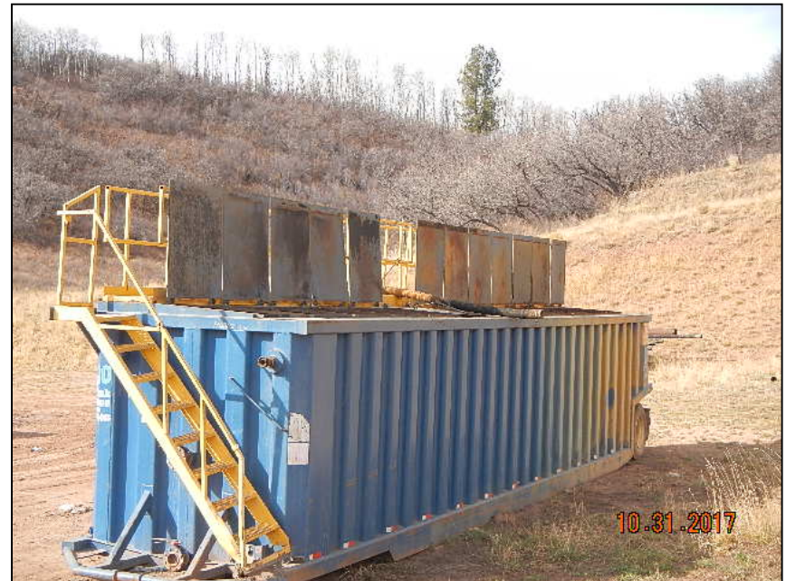
Photo 6. Hatches open at time of inspection.
