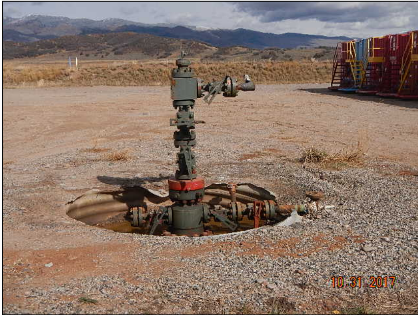
Photo 3. Wellhead has been disconnected from production.
