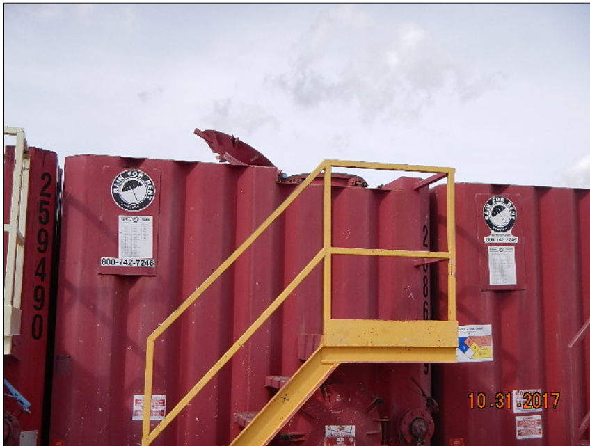
Photo 1. Hatches open on unused tanks.
