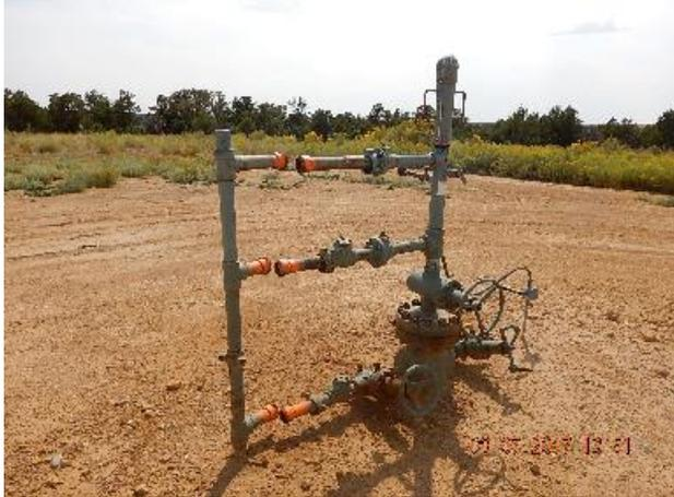
**Photo 3: Disconnected wellhead and riser previous inspection.**
