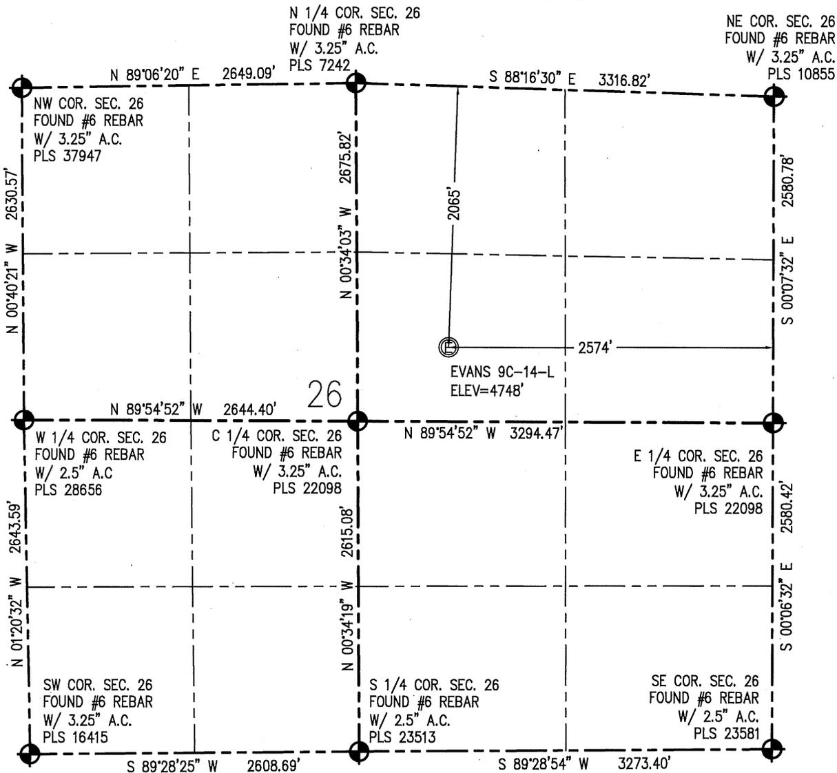
**N** IN ACCORDANCE WITH A REQUEST FROM BRANDON LORENZ - SYNERGY RESOURCES, BASELINE ENGINEERING CORP. HAS DETERMINED THE LOCATION OF THE EVANS 9C-14-L TO BE 2065' FNL AND 2574' FEL, AS MEASURED AT NINETY (90) DEGREES FROM THE SECTION LINE OF SECTION 26, TOWNSHIP 5 NORTH, RANGE 66 WEST, 6TH PRINCIPAL MERIDIAN, WELD COUNTY, COLORADO.
