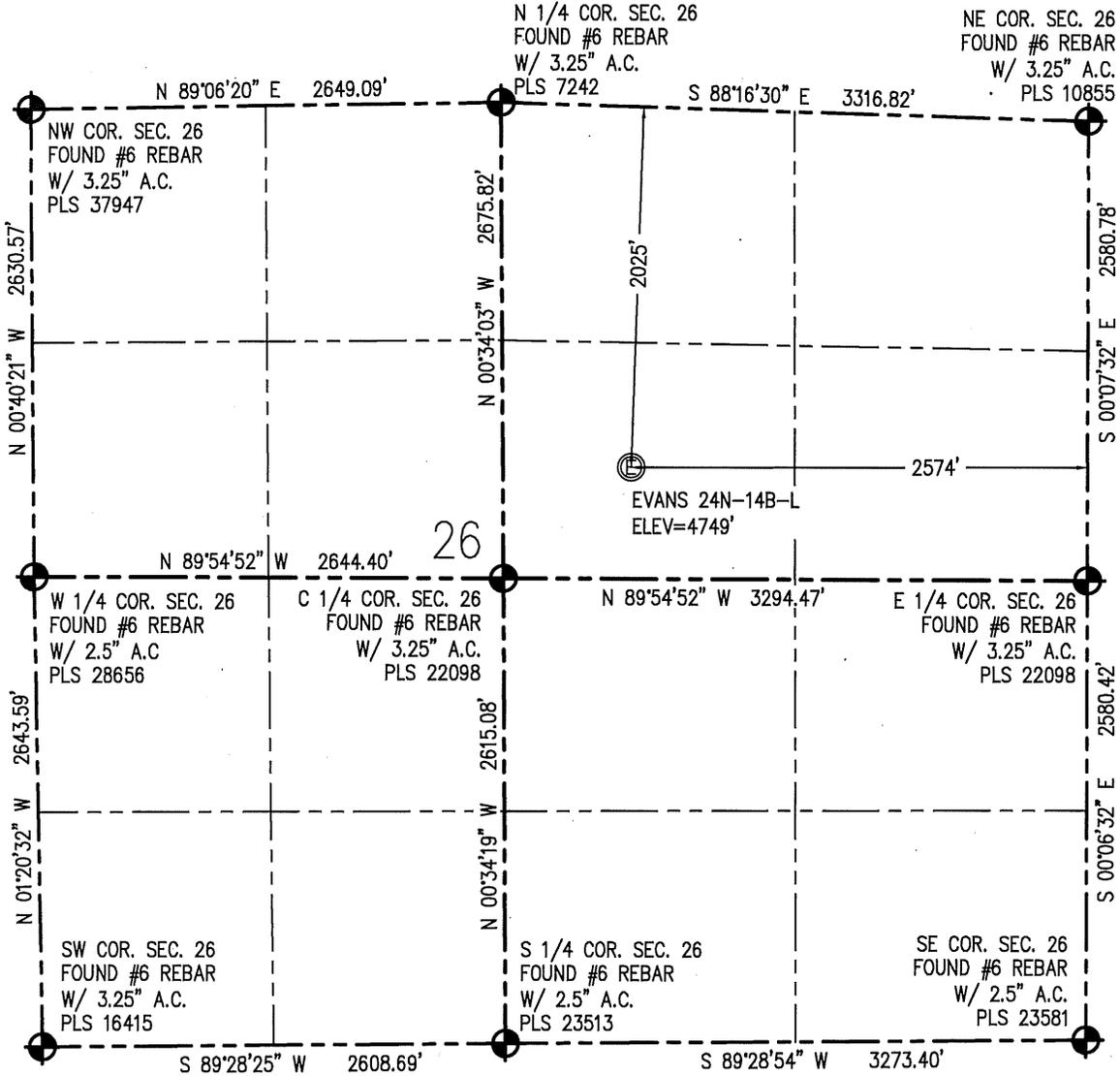
**N** IN ACCORDANCE WITH A REQUEST FROM BRANDON LORENZ - SYNERGY RESOURCES, BASELINE ENGINEERING CORP. HAS DETERMINED THE LOCATION OF THE EVANS 24N-14B-L TO BE 2025' FNL AND 2574' FEL, AS MEASURED AT NINETY (90) DEGREES FROM THE SECTION LINE OF SECTION 26, TOWNSHIP 5 NORTH, RANGE 66 WEST, WELD COUNTY, COLORADO.
