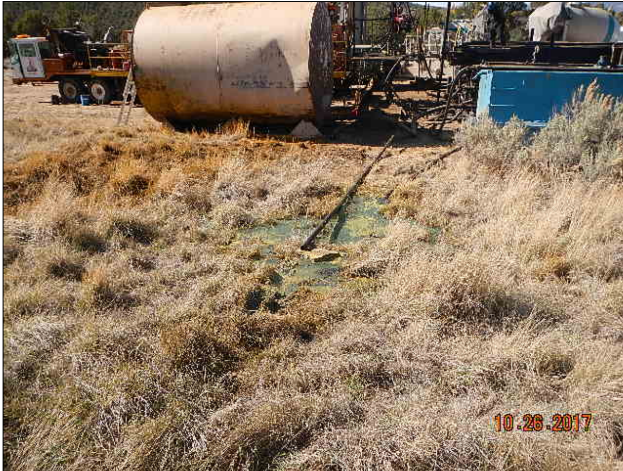
Photo 3. Paraffin pooling on East side of wellhead.
