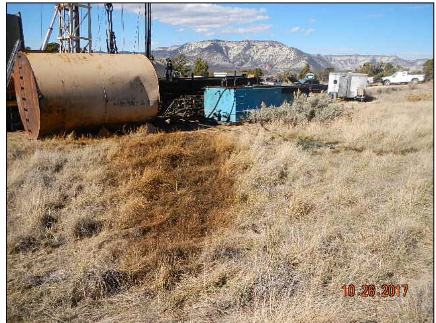
Photo 2. Paraffin staining East of wellhead.
