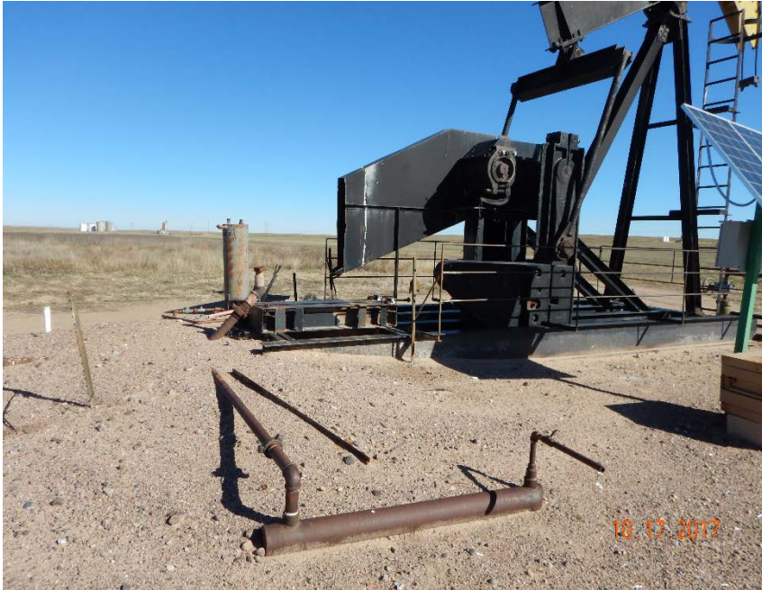
Photo #3 – Disassembled pump jack suggests that well may be incapable of production, although well is equipped with a plunger lift.
