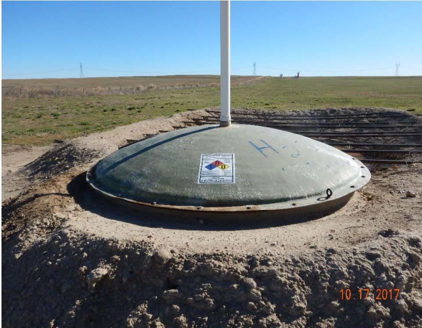
Photo #29 – Skim tank inside of pit berm at NE corner of production facility lacks berms of its own.
