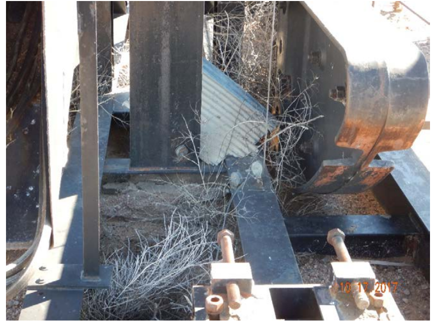
Photo #4 – Accumulation of debris and wind-blown weeds beneath pump jack.
