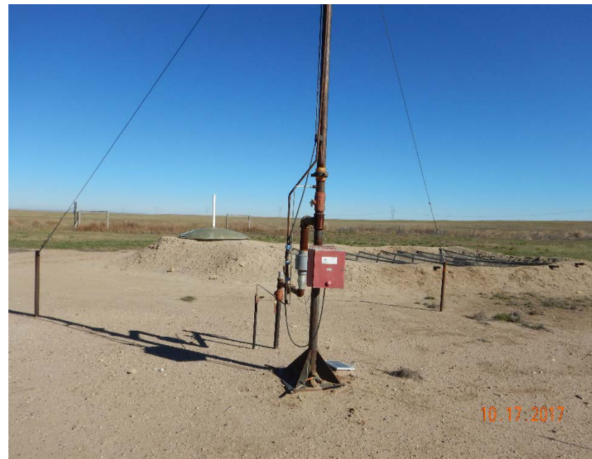
Photo #36 – Close-up view of flare control box and associated flowlines.
