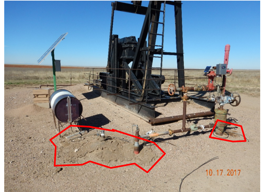
Photo #2 – Historical accumulations of oil-stained soil beneath wellhead, day tank, and flowline riser at SE corner of pump jack. Note: day tank lacking secondary containment device.
