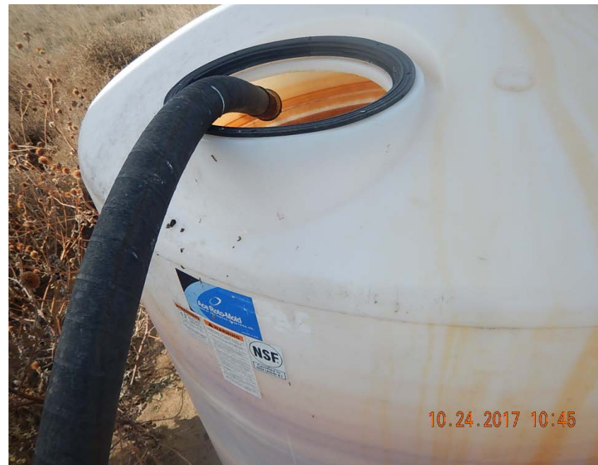
Photo 12: Open produced water tank
