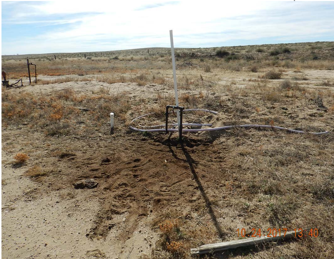
Stained soil around piping. Soil had strong hydrocarbon odor.
