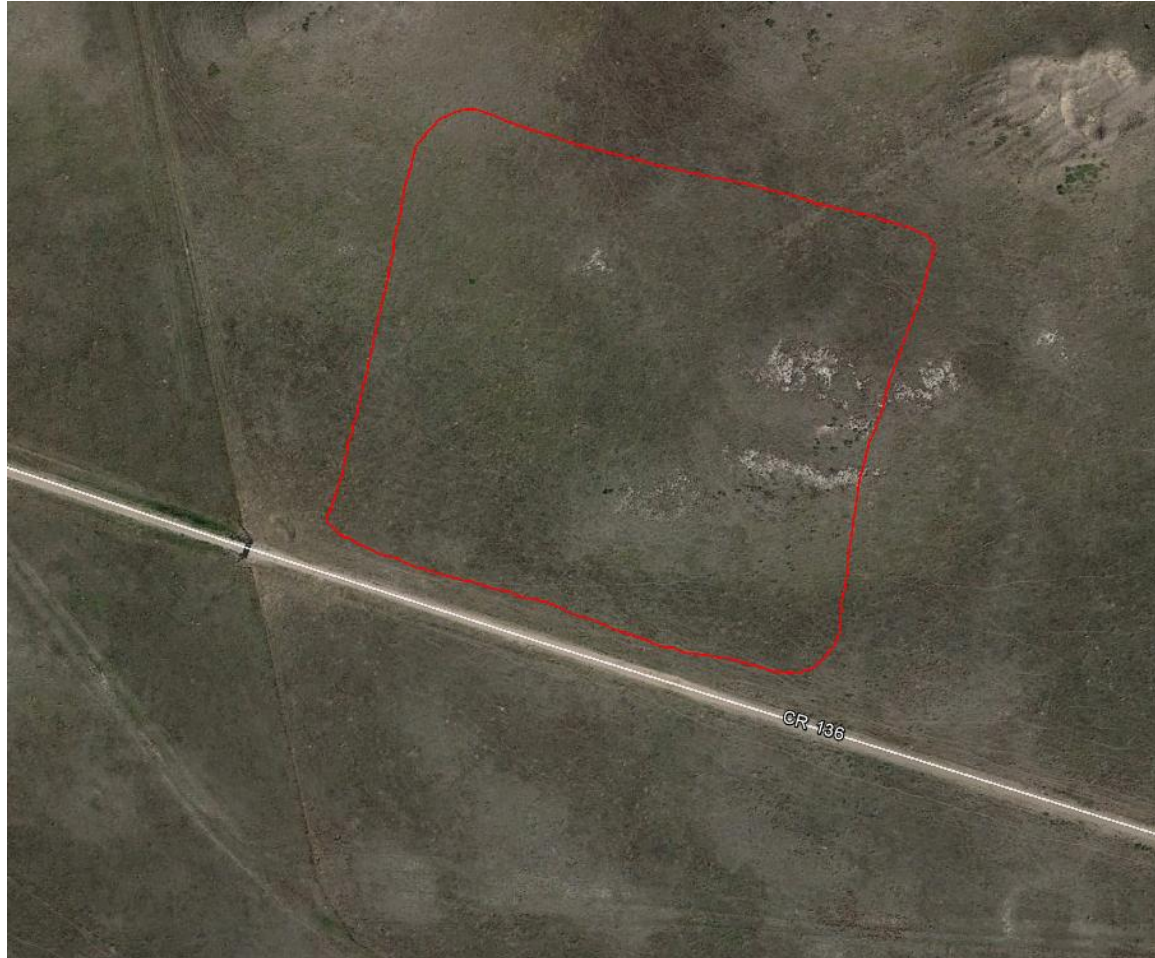
Photo 1. Google Earth aerial imagery taken on September 7, 2016. A disturbance area of 8.95 acres was mapped on 10/24/2017 using a Trimble Juno 3B handheld device (red line). Appears the Operator has overbuilt the location by 1.55 acres (21% overbuilt) per the approved Form 2A .
