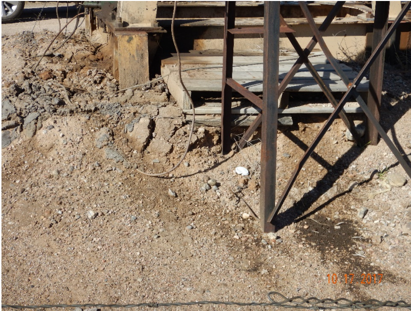
Photo #3 – Localized, oil-stained soil beneath south end of pump jack and beneath day tank at SE corner of pump jack.
