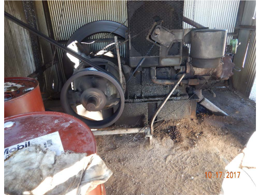
Photo #4 – Localized, oil-stained soil beneath prime mover. Also pictured: chemical storage drums inside of shed.
