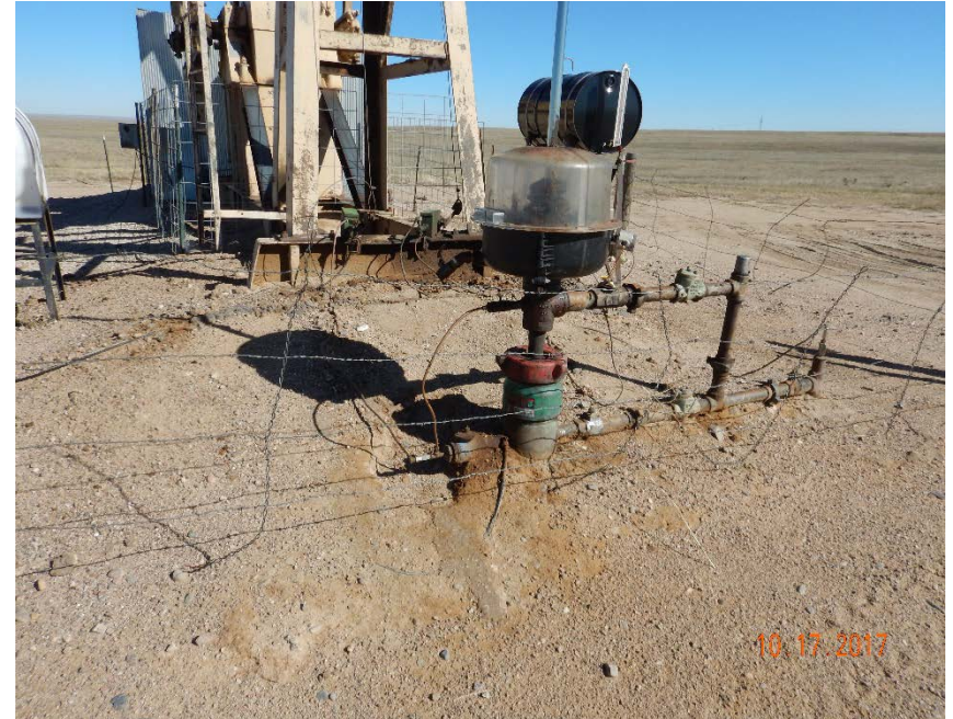
Photo #2 – Oil-stained soil accumulation at wellhead (foreground) and SE corner of pump jack (background).
