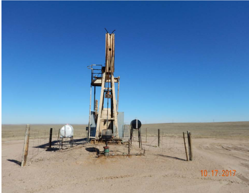
Photo #1 – View of wellhead and pump jack from the south. Note chemical storage containers on either side of pump jack lack secondary containment devices.
