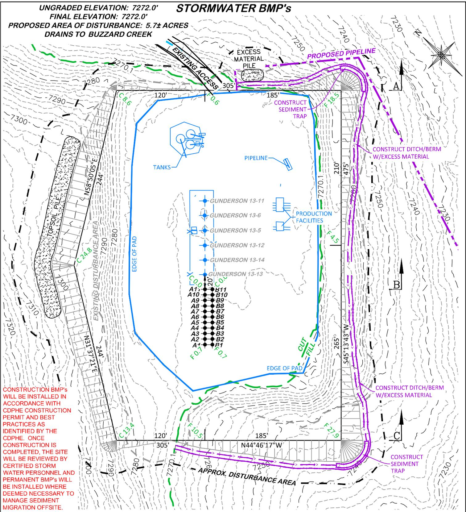
CONSTRUCTION BMP's WILL BE INSTALLED IN ACCORDANCE WITH CDPHE CONSTRUCTION PERMIT AND BEST PRACTICES AS IDENTIFIED BY THE CDPHE. ONCE CONSTRUCTION IS COMPLETED, THE SITE WILL BE REVIEWED BY CERTIFIED STORM WATER PERSONNEL AND PERMANENT BMP's WILL BE INSTALLED WHERE DEEMED NECESSARY TO MANAGE SEDIMENT MIGRATION OFFSITE.
