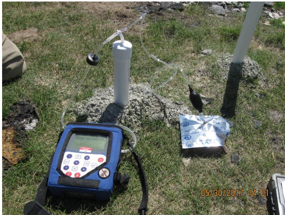
Vent well sampling setup showing Landtec GEM being used to purge well and screen soil gas readings, and Cali-5-Bond gas sampling bag connected with squeeze bulb pump.
