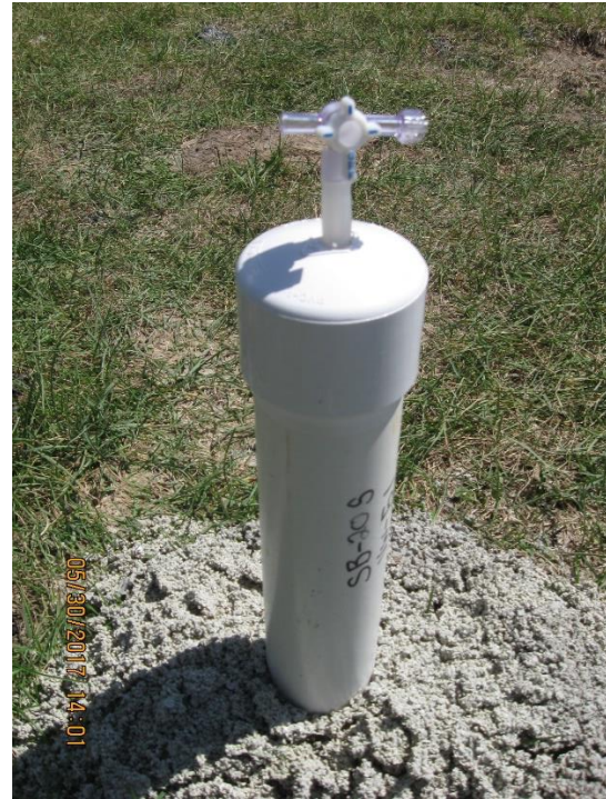
Typical soil gas monitor well stick-up showing addition of slip cap, Teflon seal, polyethylene drop tube, silicone tubing through cap, and 3-way valve in the closed position.
