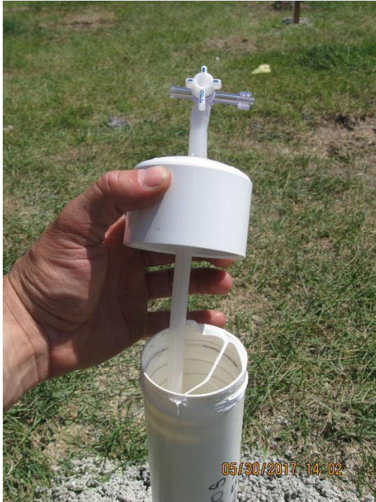
Typical soil gas monitor well stick-up showing addition of slip cap, Teflon seal, polyethylene drop tube, silicone tubing through cap, and 3-way valve in the closed position.
