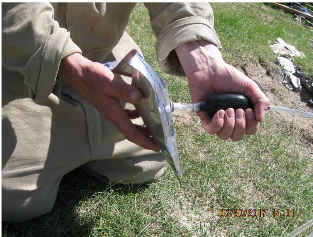
Filling a Cali-5-Bond gas sampling bag with soil gas using squeeze bulb pump.
