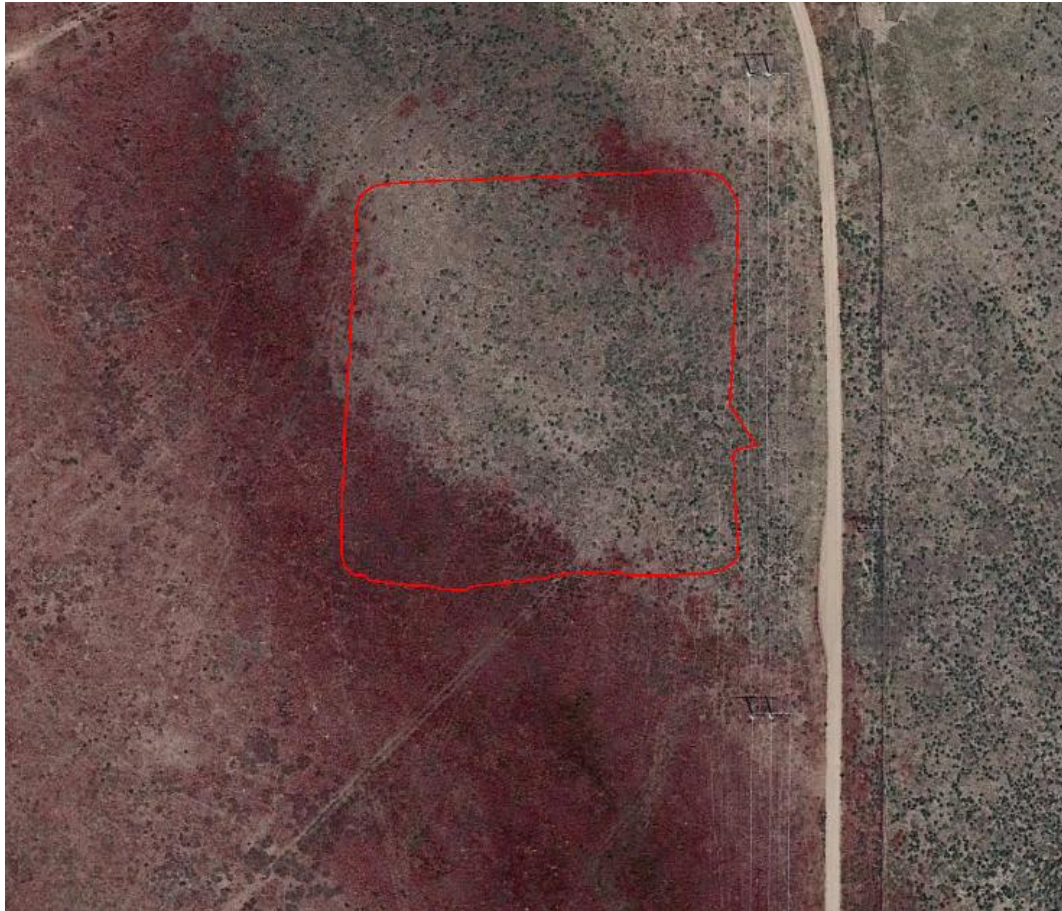
Photo 1. Google Earth aerial imagery taken on June 14, 2016. A disturbance area of 4.64 acres was mapped on 10/12/2017 using a Trimble Juno 3B handheld device (red line). Appears the Operator has overbuilt the location by 0.94 acres (25% overbuilt) per the approved Form 2A .
