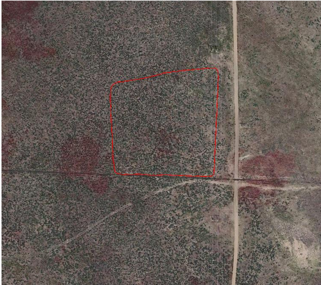
Photo 1. Google Earth aerial imagery taken on June 14, 2016. A disturbance area of 4.75 acres was mapped on 10/12/2017 using a Trimble Juno 3B handheld device (red line). Appears the Operator has overbuilt the location by 1.25 acres (36% overbuilt) per the approved Form 2A .
