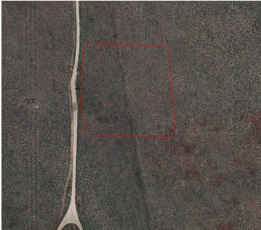
Photo 1. Google Earth aerial imagery taken on June 14, 2016. A disturbance area of 4.33 acres was mapped on 10/12/2017 using a Trimble Juno 3B handheld device (red line). Appears the Operator has overbuilt the location by 1.23 acres (40% overbuilt) per the approved Form 2A .
