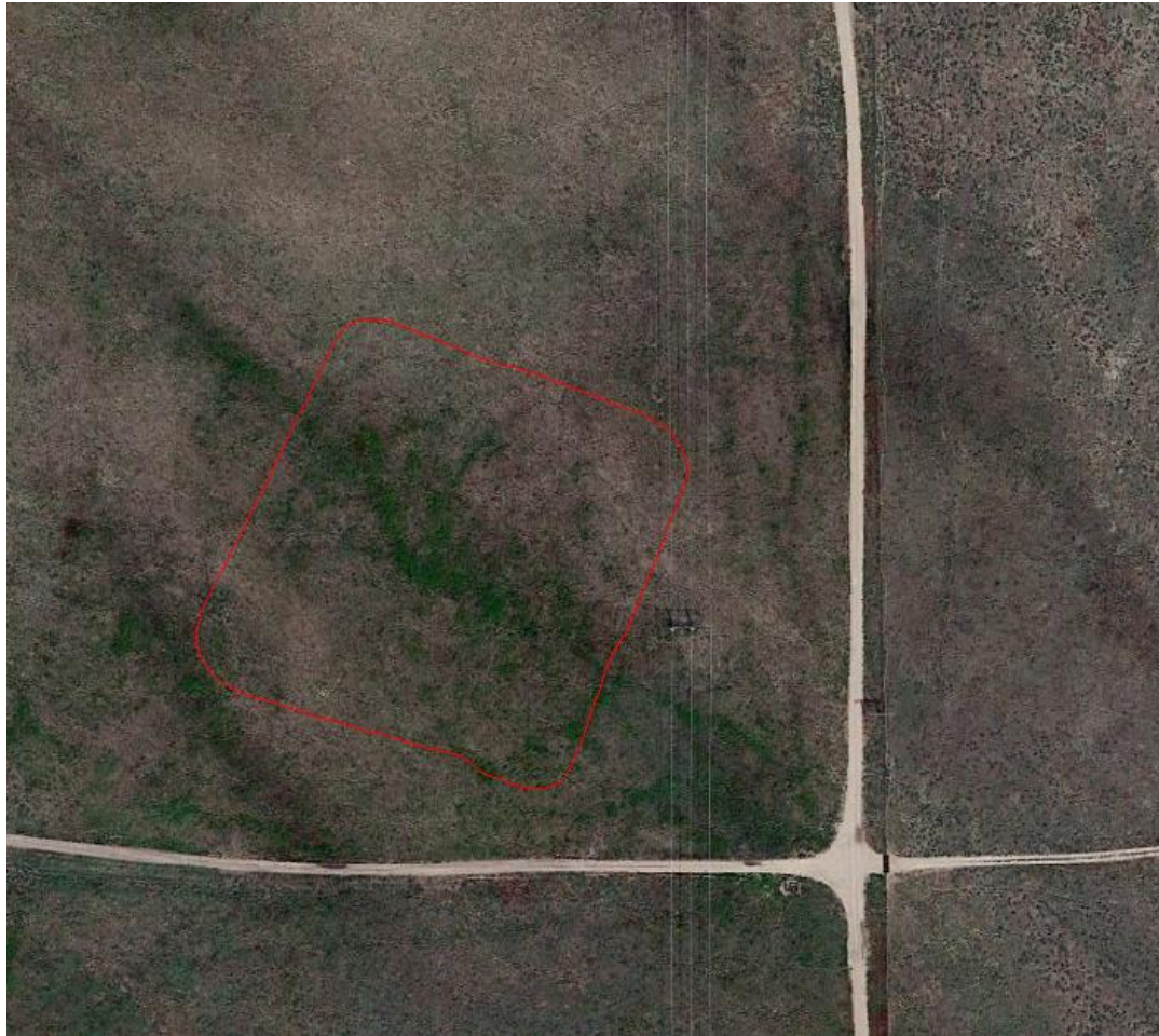
Photo 1. Google Earth aerial imagery taken on June 14, 2016. A disturbance area of 4.53 acres was mapped on 10/12/2017 using a Trimble Juno 3B handheld device (red line). Appears the Operator has overbuilt the location by 1.43 acres (46% overbuilt) per the approved Form 2A .
