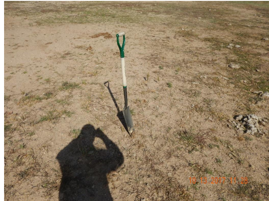
Photo 6: Photo taken from the location. Inspector had tested the site for compaction concerns. Photo shows inspector was only able to penetrate the first couple of inches of topsoil with relative ease.
