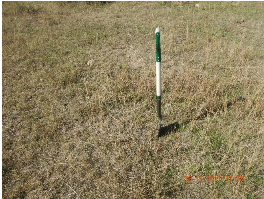
Photo 7: Photo taken from the reference area. Inspector had tested the soil in the reference area for comparison to that of the disturbance area. Photo shows inspector was able to easily penetrate the topsoil.
