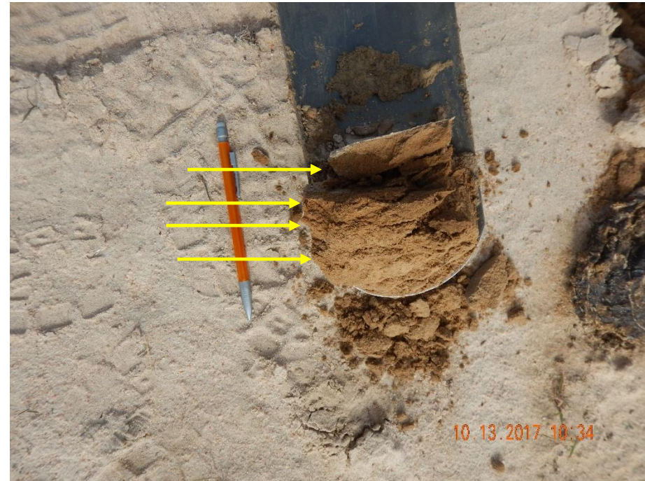
Photo 12: Inspector tested the site for soil compaction, photo shows horizontal plate formations in the top inches of soil. This is an indication of soil compaction.
