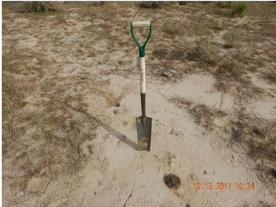
Photo 11: Photo taken from the location. Inspector had tested the site for compaction concerns. Photo shows inspector was only able to penetrate the first couple of inches of topsoil with relative ease.
