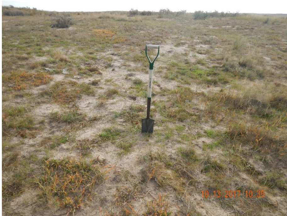
Photo 13: Photo taken from the reference area. Inspector had tested the soil in the reference area for comparison. Photo shows inspector was able to easily penetrate the topsoil.
