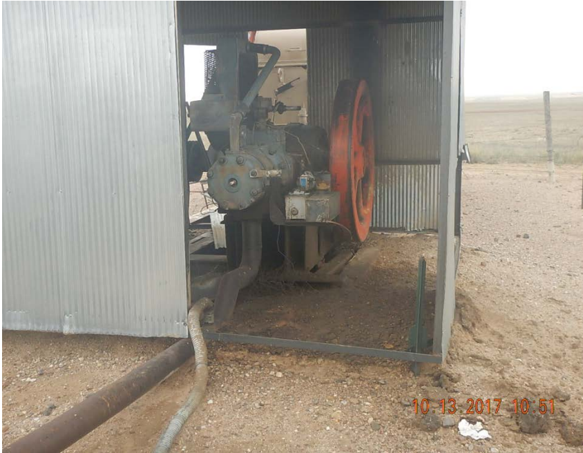
Photo 3: Stained soil at engine
