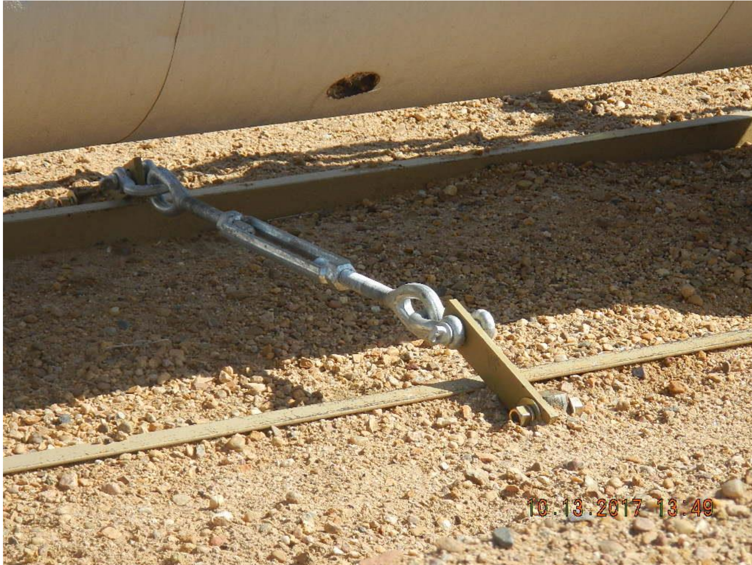
Flood Anchor on Separator Location Number: 421051
