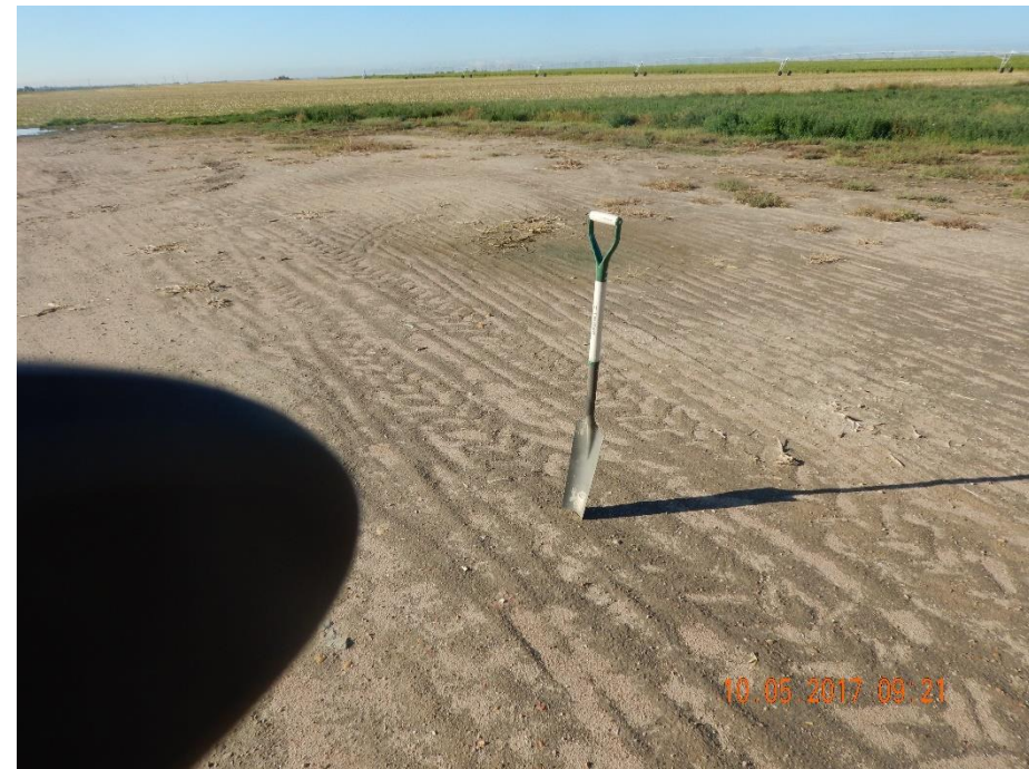
Photo 3: Photo taken from the former battery location. Photo shows inspector had tested the location to see if compaction concerns remains. Photo shows that the shovel was only able to penetrate the first couple of inches with ease. Compaction concerns remain.
