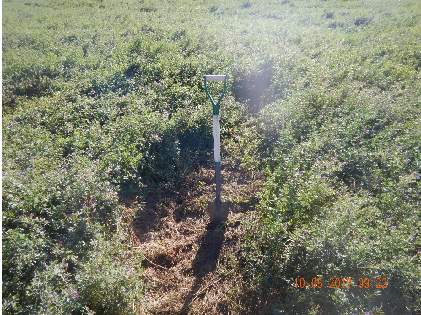
Photo 4: Photo taken from the adjacent reference area. Inspector had tested the soil in the reference area to compare to the disturbance area. Inspector was able to penetrate ~10 inches of topsoil without difficulty.
