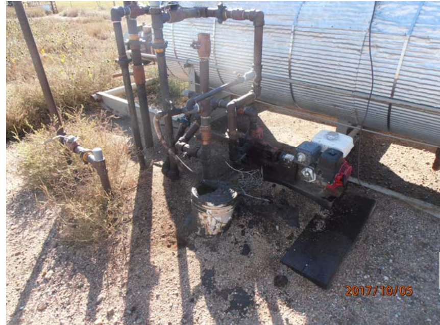
Photo 4: Oily soil at pump adjacent flowlines and horizontal separator.
