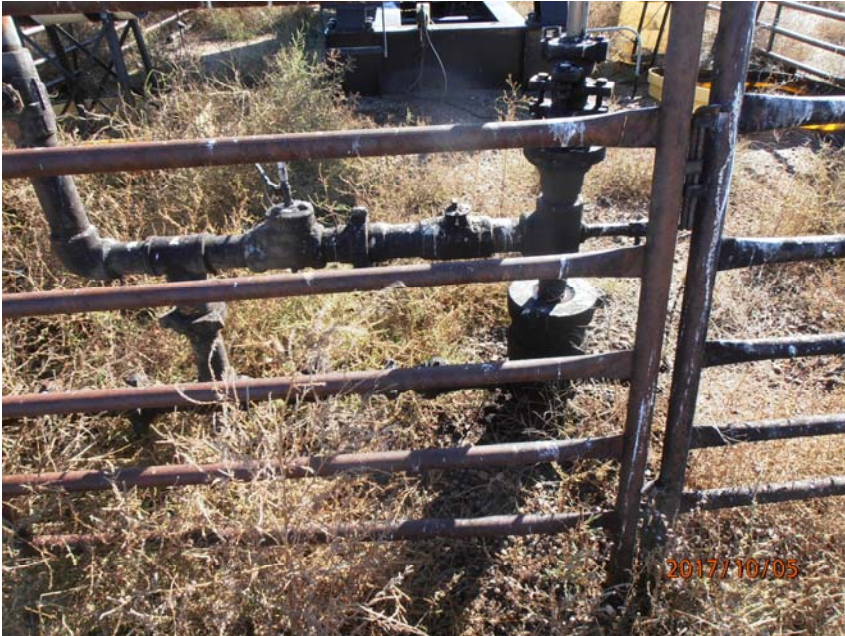
Photo 7: Oily soil at wellhead.
