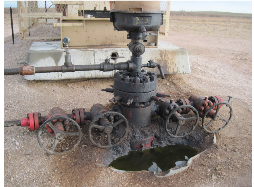
STAINED SOIL AROUND WELLHEAD
