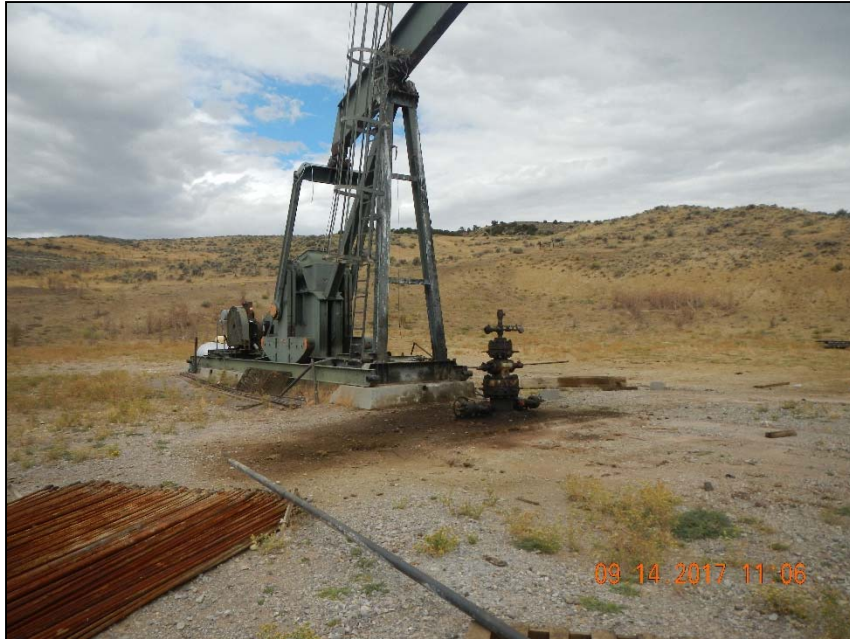
Photo 3. Stained soil at wellhead.
