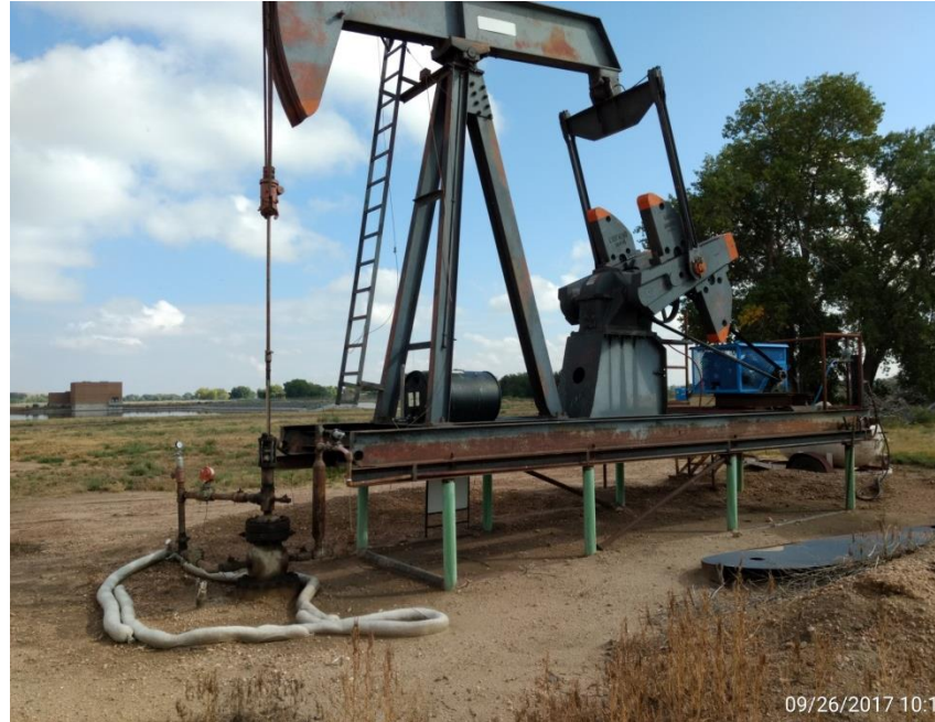
Wellhead, Pumping unit, and prime mover
