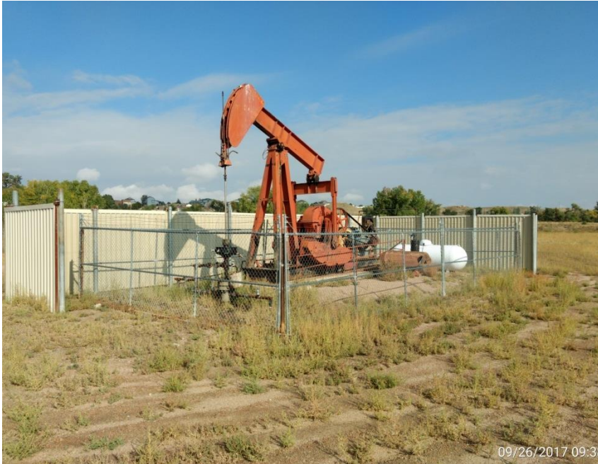
Wellhead, pumping unit, and prime mover
