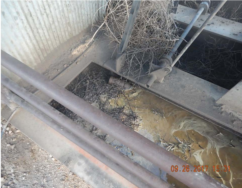
Photo 9: Stained soil, oily fluid at pump jack
