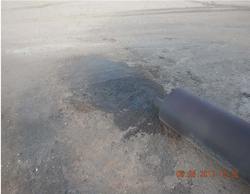
Photo 11: Stained soil at ajax exhaust
