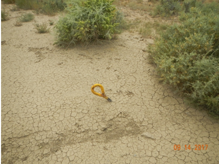
Photo 5: View of rig anchor still present within the project area. All rig anchors need to be removed.
