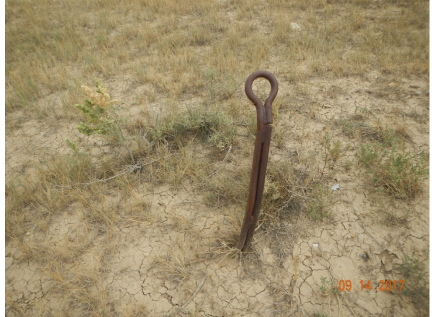
Photo 6: View of riser near the entrance to the well pad needing to be removed.
