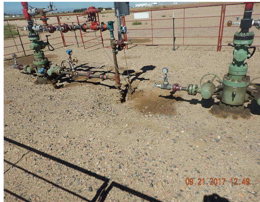
Photo 6: Stained soil at Wellheads on W side.
