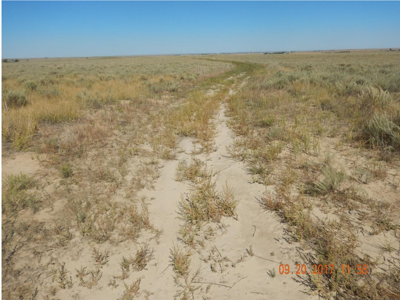
Photo 3: Photo taken from the north end of the location, facing north. Photo shows access road has not been reclaimed in accordance to COGCC 1000 series requirements.
