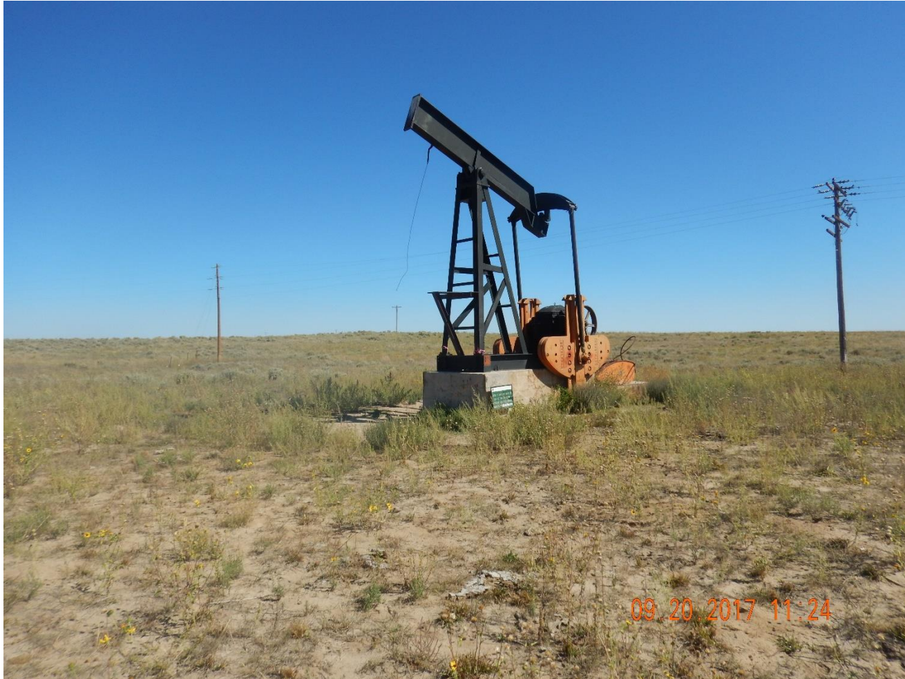
Photo 1: Photo shows pump unit and base has not been removed per the corrective action.
