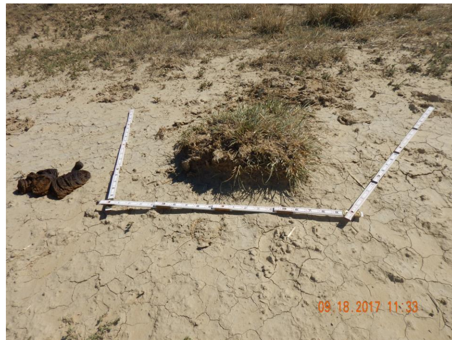
Photo 4: Photo taken from the northern degradation area. Photo shows pedestal formations occurring due to stormwater degradation. Pedestals form when stormwater (or wind erosion) erodes away un-stabilized areas of soil around vegetation.
